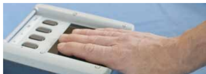
Taking flat impressions of 4 fingers with PAPILLON DS-30N
